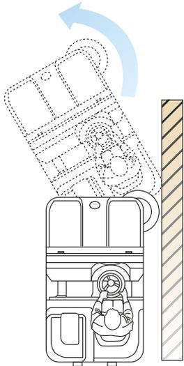
The body with rounded edges and protected by a rubber profile improves sweeper manoeuvrability
