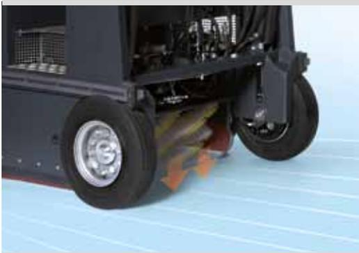
The central brush is the floating type and self-adjusts to keep in contact with the ground all the time
